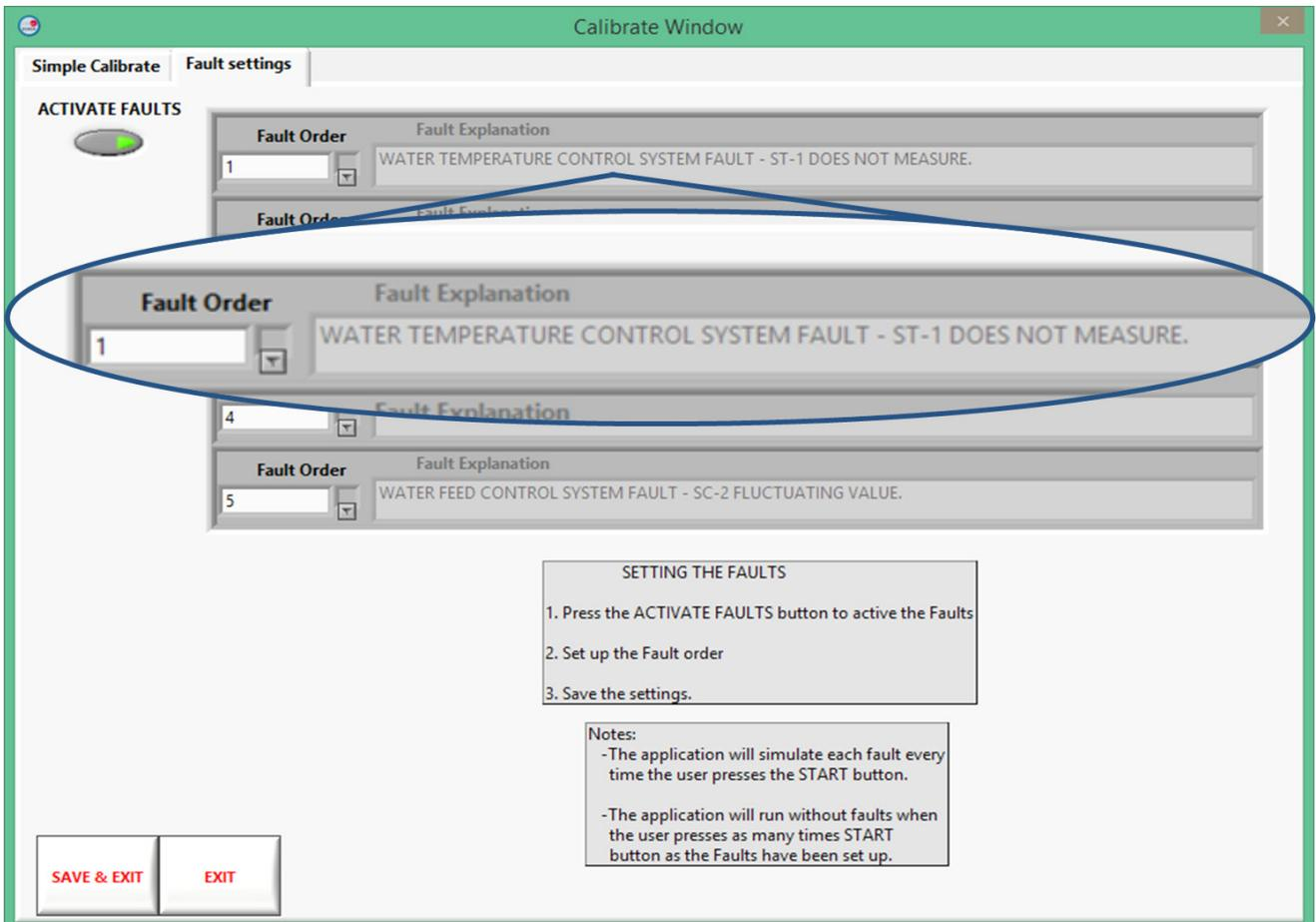
Single fault execution example, consisting on an anomalous temperature measurement. The student must determine the causes of such anomaly as well as deciding the most appropriate corrective actions to fix that fault
