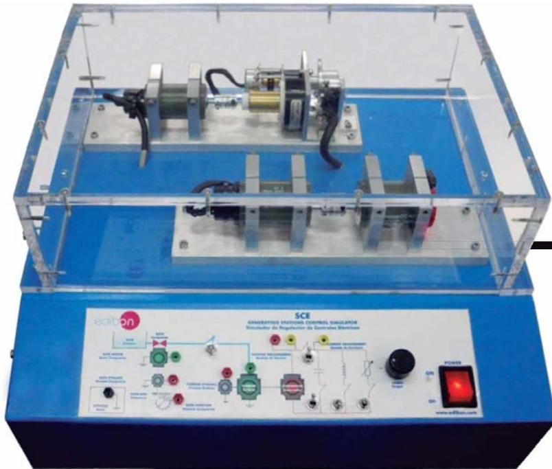
① Unit: SCE. Generating Stations Control and Regulation Simulator, including control interface
