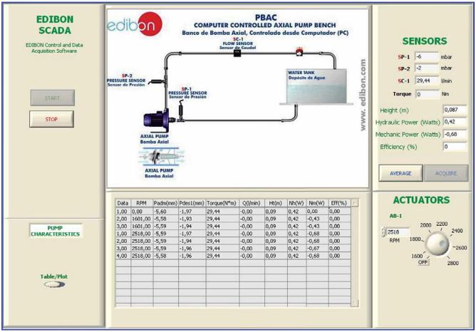
The software allows the plotting of the characteristic curves of the Axial Pump and their comparison with the theoretical working curves.
