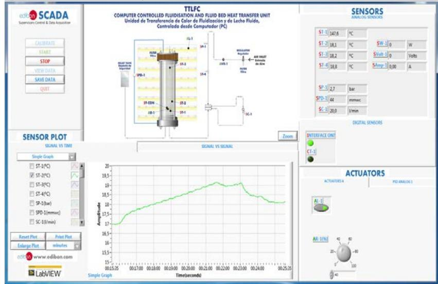
Representation in real time of the measured magnitudes. Temperature profile in a fluidized bed (particles 170 – 300 microns).
