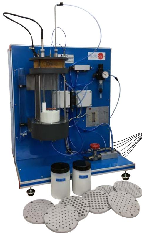
① Unit: TTLFC. Computer Controlled Fluidization and Fluid Bed Heat Transfer Unit
