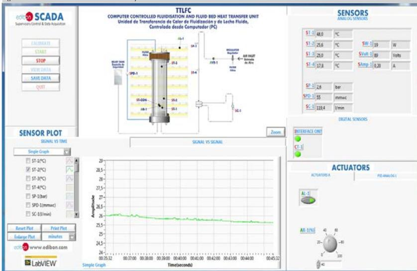
The heating temperature control is done through a PID control. When the target temperature is reached at the temperature sensor (ST-1), the heating element is turned off.
