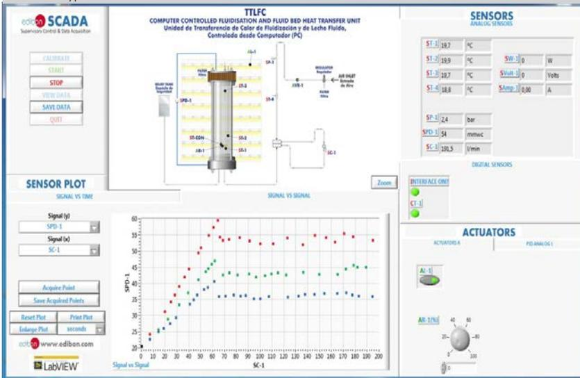
Representation in real time of the measured magnitudes. Fluidization with different particle size.
