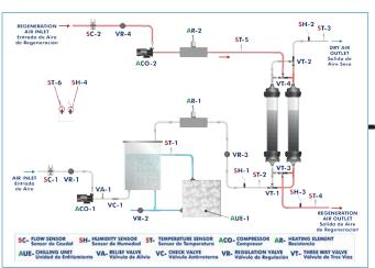
Unit: QSAC. Computer Controlled Adsorptive Air Drying Unit
