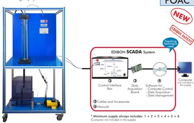
1 Unit: POAC Computer Controlled Advanced Oxidation Unit
