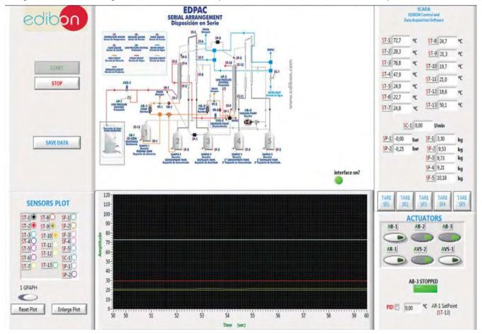
Double-effect arrangement: the steam generated in the first column is used to heat, being it introduced in the jacket of the second column. The screen below allows to observe how a PID control for the heating element is done, fixing the temperature of the food to be introduced in the column to 60°C.
