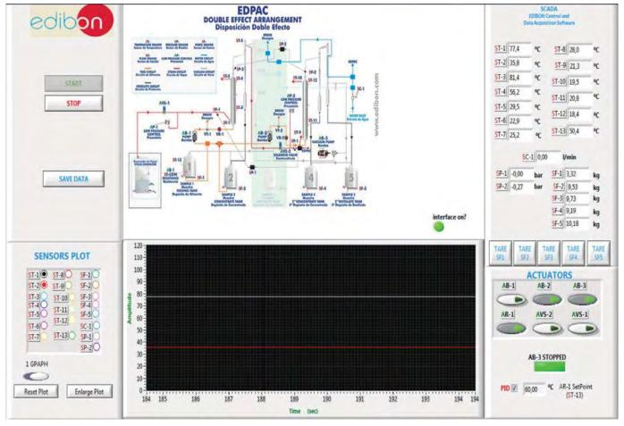
The optional accessory EDPDC must be connected to the corresponding intakes of the EDPAC unit. The sensors are extracted from the EDPAC unit in function of the measurements under study. The software allows to select the sensors under operation for an easy reading and plotting.
