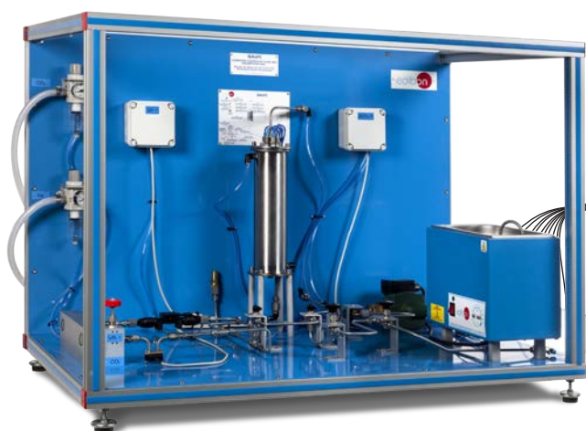
① Unit: QALFC. Computer Controlled Fixed Bed Adsorption Unit
