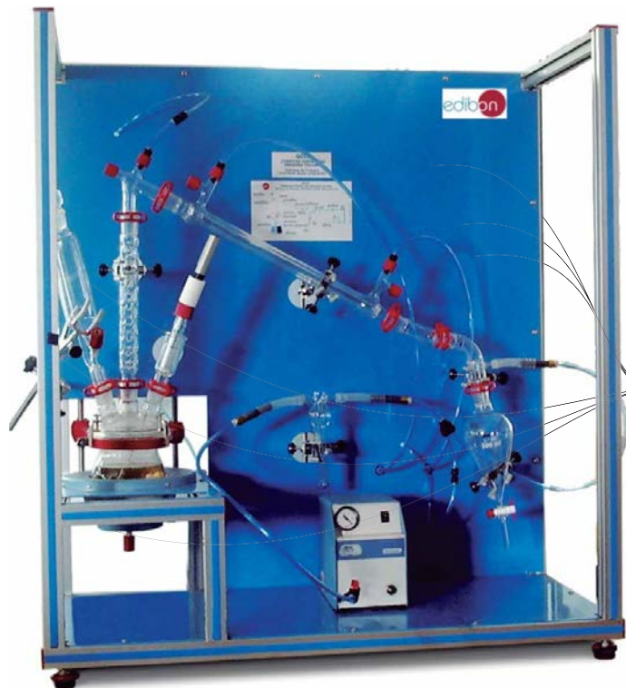
① Unit: QCCC. Cracking Column
