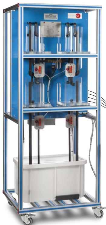
① Unit: CTAC. Computer Controlled Coupled Tanks System
