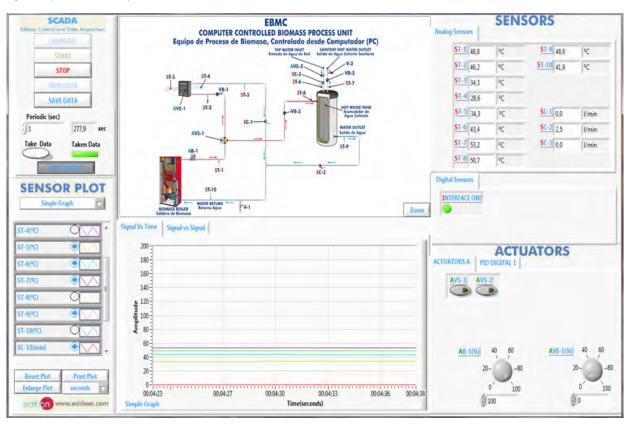
When the solenoid valve (AVS-1) is activated, the heating water can go towards both primary circuits and the flow can be regulated from 0 to 100% (AB-1 pump).
