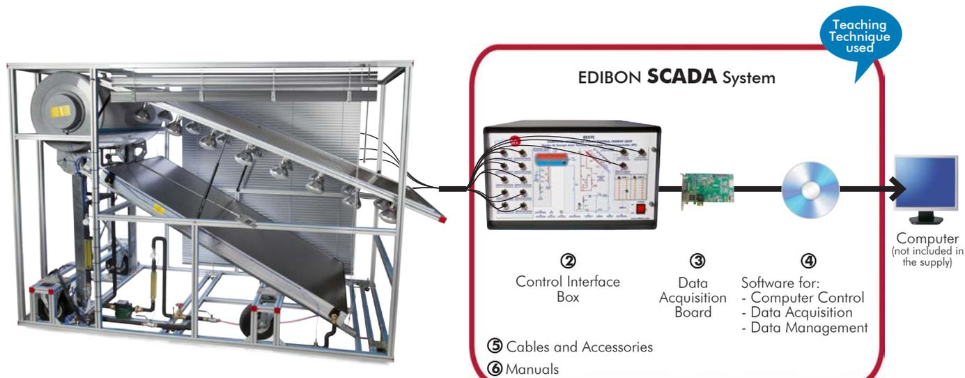
① Unit: EESTC. Computer Controlled Thermal Solar Energy Unit
