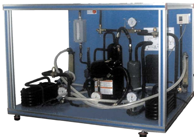
① Unit: THBLLC. Computer Controlled Heat Pump Unit (one condenser (water) and one evaporator (water))
