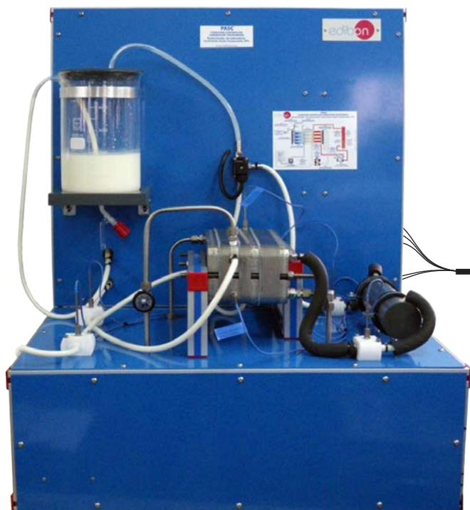
① Unit: PASC. Computer Controlled Laboratory Pasteurizer
