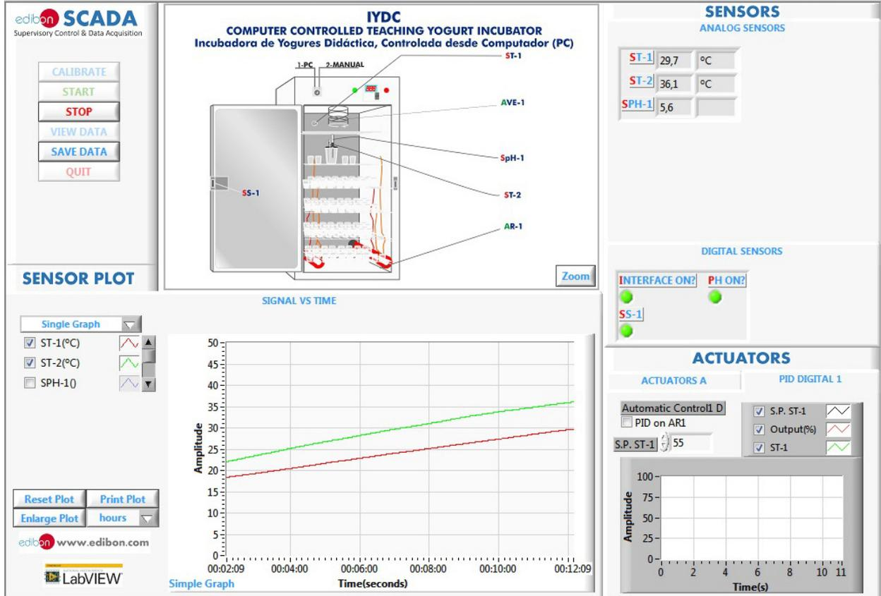
Representation in real time of the measured magnitudes. Graphs with pH and temperature measures visualization.
