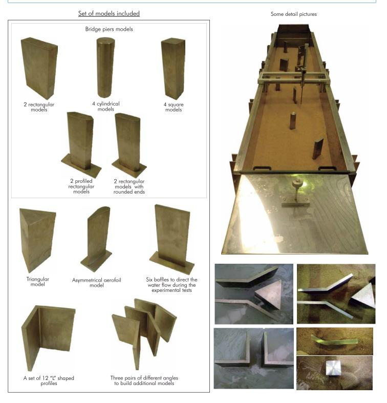
The Mobile Bed and Flow Visualization Unit (HVFLM-4) is mounted on a metallic structure with wheels, rigid and resistance enough to support the weight of water and sand without suffering any deformation. All components in contact with water are of non-corrosive materials. The unit includes a diagram with similar distribution to the elements in the real unit.
