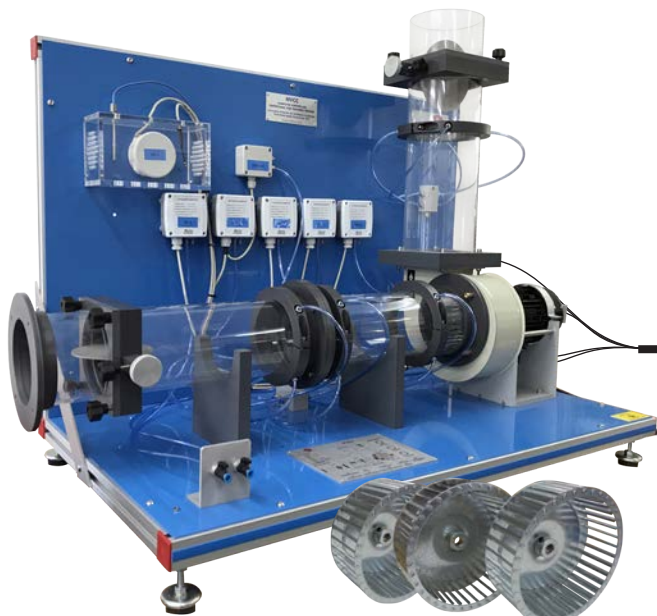
Detail of the set of turbines supplied with the units
