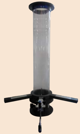
HVCC-CTPG. 114 mm. diameter duct and pressure taking with Pitot
