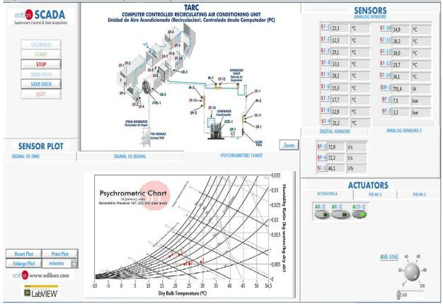
Heating temperature control is done through a PID control. When the target temperature is reached at the temperature sensor (ST-5), the heating element AR-2 is turned off.
