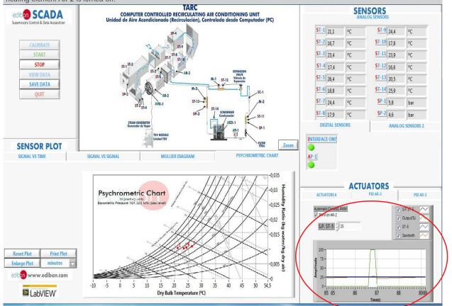
Heating temperature control is done through a PID control. When the target temperature is reached at the temperature sensor (ST-9), the heating element AR-3 is turned off.
