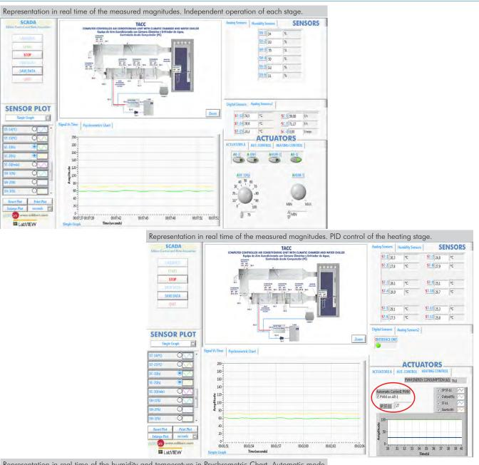
Representation in real time of the humidity and temperature in Psychrometric Chart. Automatic mode setting confort in the climatic chamber.
