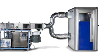
0 Unit: TACC. Computer Controlled Air Conditioning Unit with Climatic Chamber and Water Chiller
