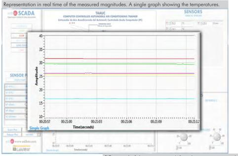
$\mathsf{PID}$  control of the compressor. When the set point is reached at the temperature sensor (ST-5), the compressor is turned off.
