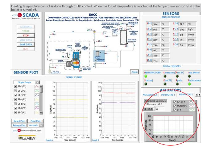
Heating temperature control is done through a PID control. When the target temperature is reached at the temperature sensor (ST-3), the boiler is turned off.
