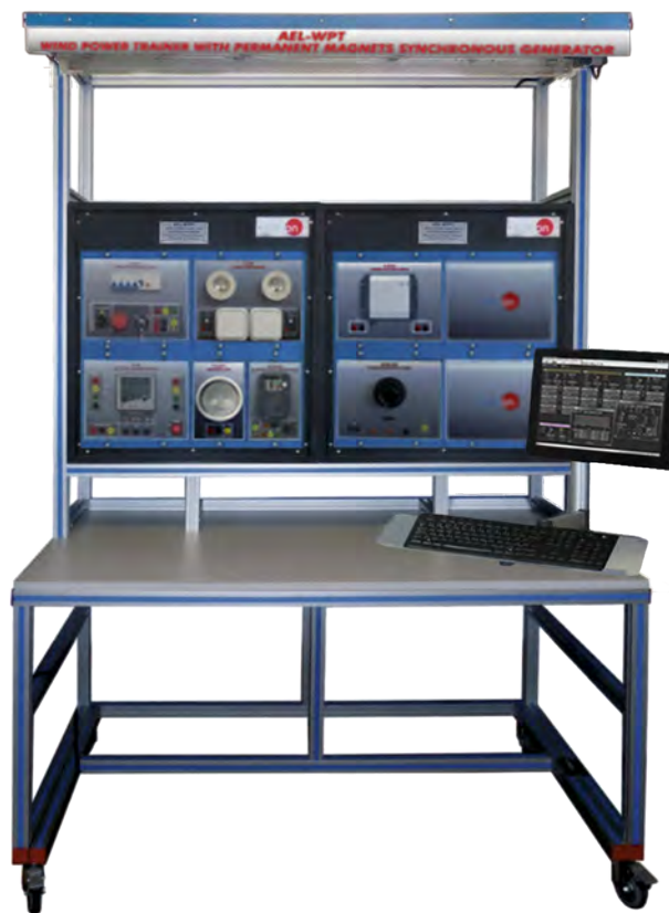
① Unit: AEL-WPT. Wind Power Application with Permanent Magnets Synchronous Generator
