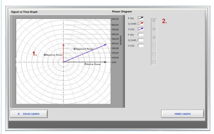
(1) Real time graph. It displays the variables selected. This picture shows the phasors diagram of the active, reactive and apparent powers of the network analyzers.
