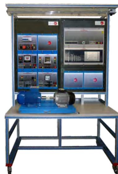
AEL-WPT. **Wind Power Trainer with Permanent Magnets Synchronous Generator** (continuation)
