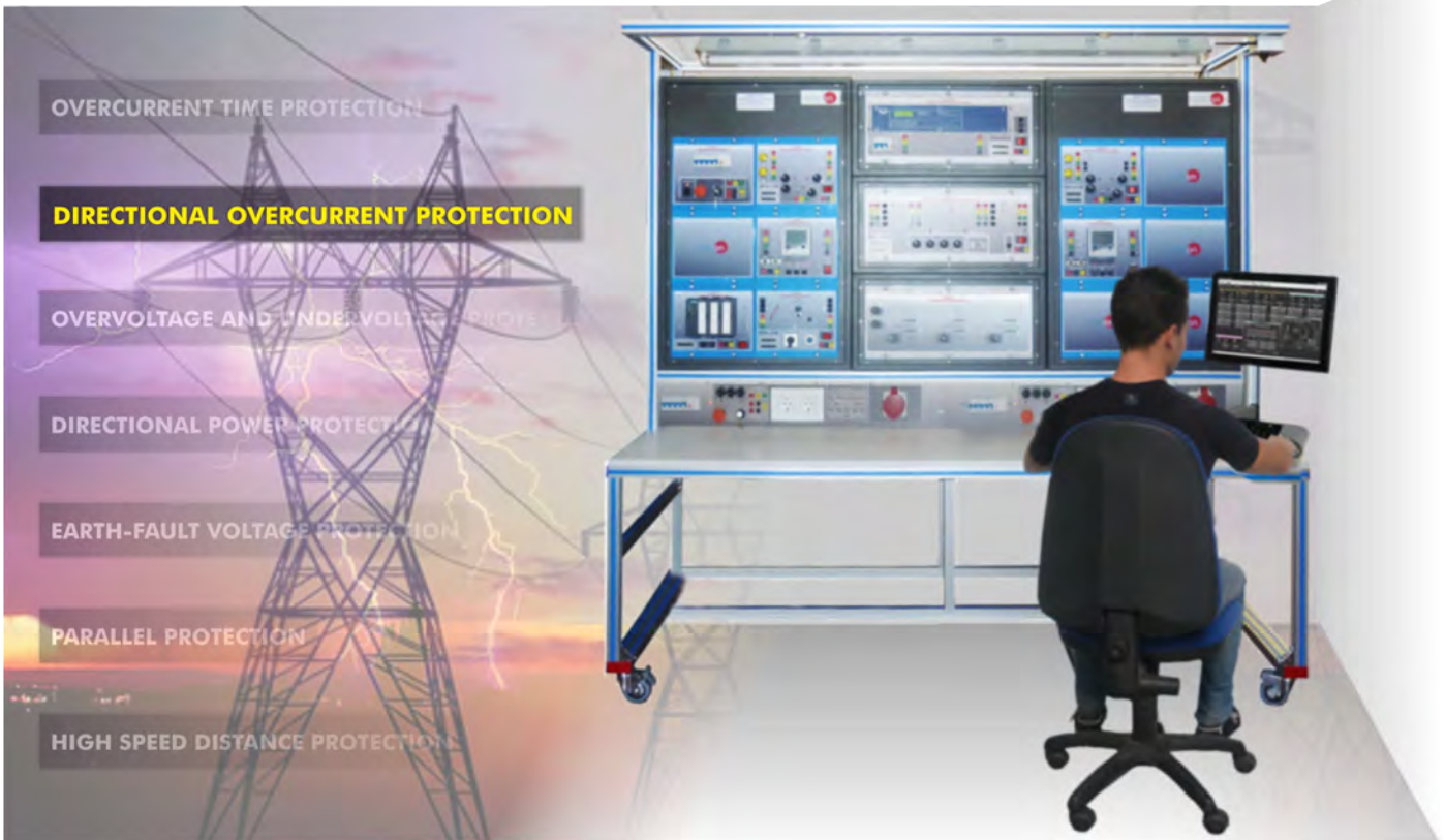
① Unit: AEL-TPT-02. Directional Overcurrent Protection for Transmission Lines
