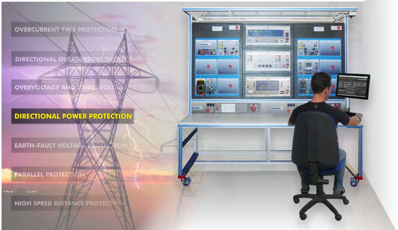
① Unit: AEL-TPT-04. Directional Power Protection Relay.
