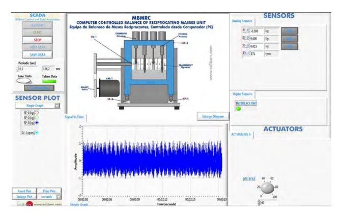
This last screen shows the data collected by the force sensors (SF-1, SF-2 and SF-3) versus time when the unit is working at a constant turning speed (VIEW DATA window).
