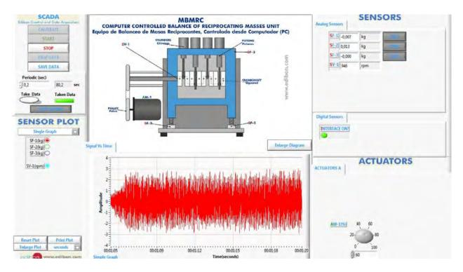
This screen shows the force (sensor SF-2) versus time when the unit is working at a constant turning speed.
