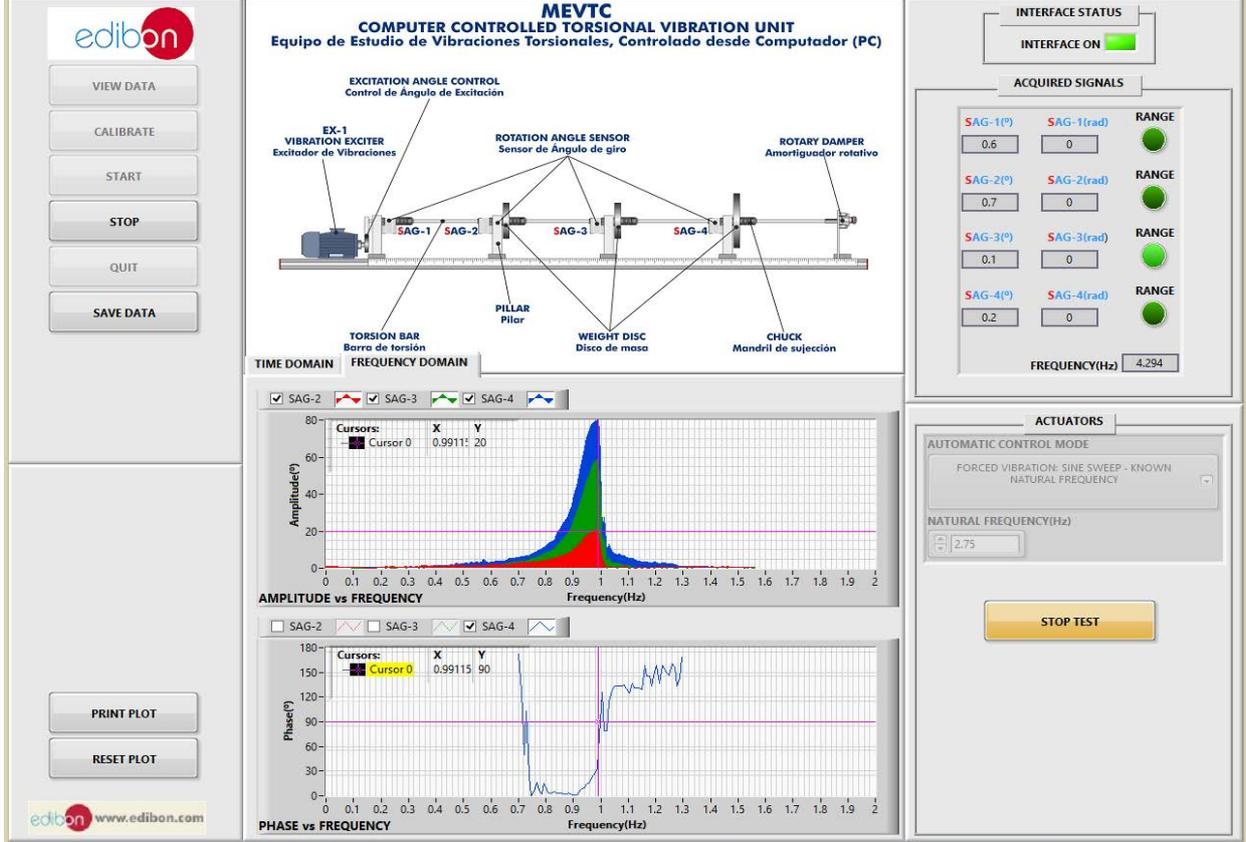
Analysis of the phase change in the natural frequency of a damped system.
