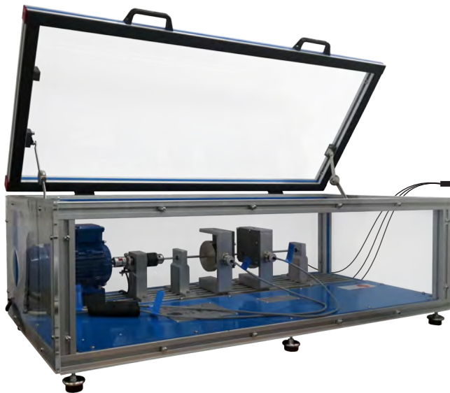
① Unit: MVCC. Computer Controlled Critical Speed Investigation Unit
