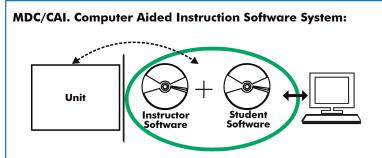
With no physical connection between unit and computer (PC), this complete software package consists of an Instructor Software (INS/SOF) totally integrated with the Student Software (MDC/SOF). Both are interconnected so that the teacher knows at any moment what is the theoretical and practical knowledge of the students.
