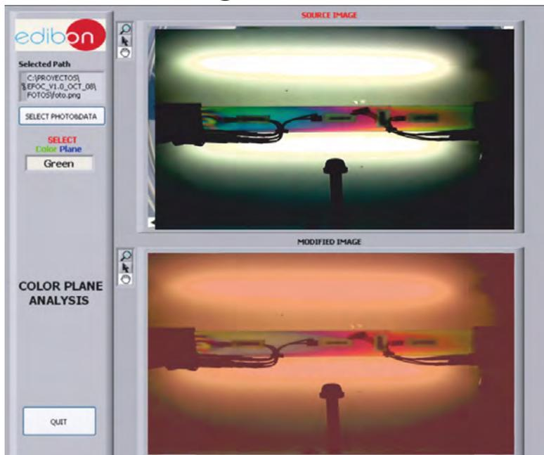
With this tool, photos captured can be analysed, extracting a specific colour component, while the experiments are being carried out.
