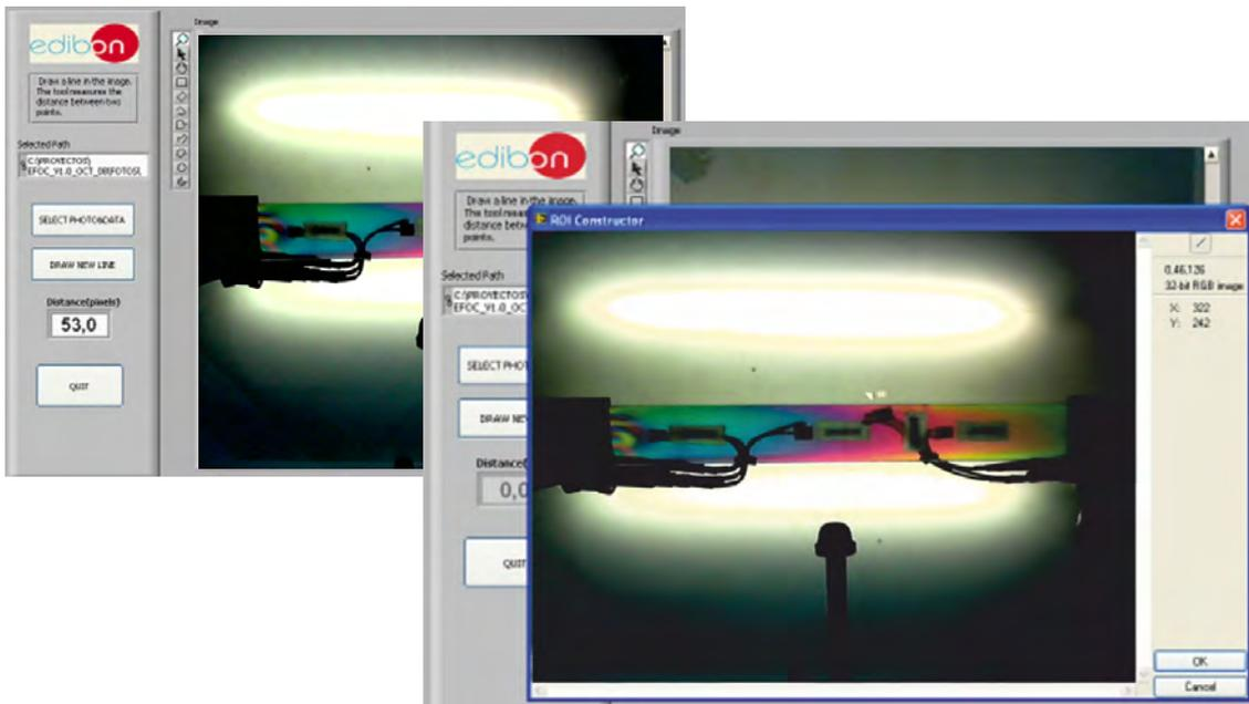
With this tool, the distance between two interest points, drawn over an image, can be quantitatively measured, while the experiments are being carried out.
