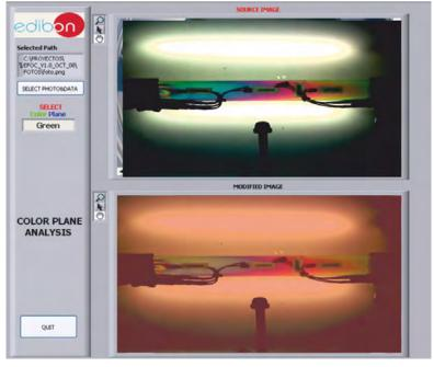
With this tool, photos captured can be analysed, extracting a specific colour component, while the experiments are being carried out.
