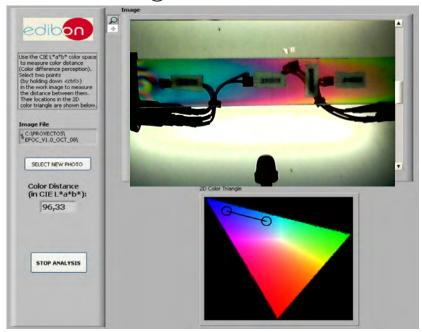
With this tool, the difference between two specific colours can be quantitatively measured, while the experiments are being carried out.
