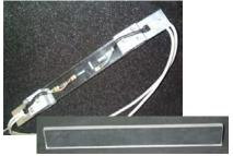
N°8-G. Big Rectangular Specimen with strain gauges + N°8 Big Rectangular Specimen
