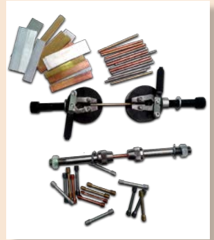
EEU/20KN-4. Tensile Tests Accessories with Standar, Flat and Round Specimens
