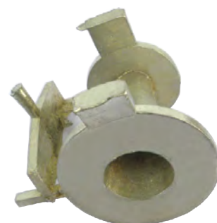
Detail of the finished casting, free of sand
