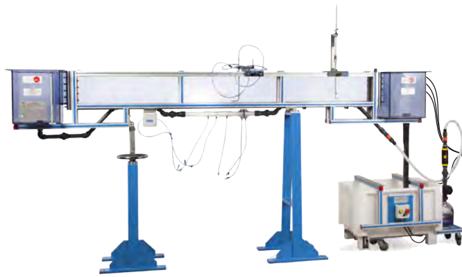
① Unit: CFC. Computer Controlled Flow Channels (section: 80 x 300 mm)
