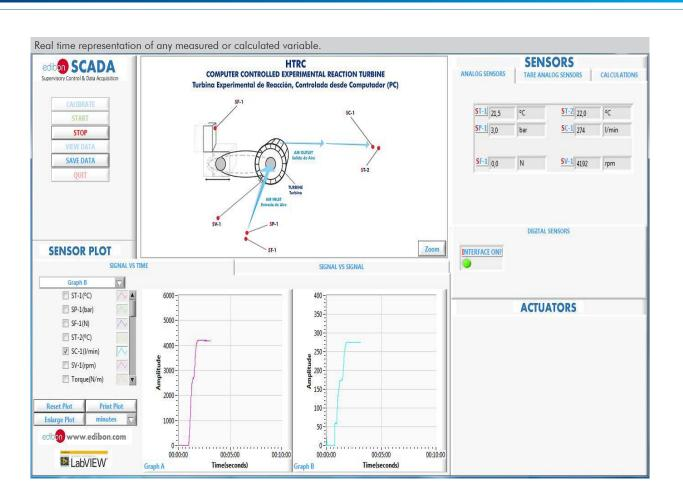
Signal versus signal chart where any of the measured or calculated variables can be represented. Mechanical power vs turbine speed.
