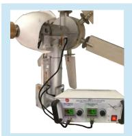
EEE/T. Force and Torque Meter for the Wind Turbine
