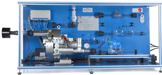
① Unit: HFCC. Computer Controlled Flow of Compressible Fluids Unit
