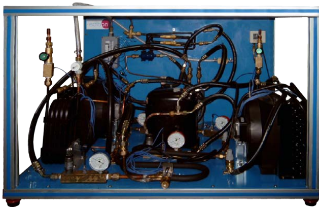
① Unit: THARA2C. Computer Controlled Refrigeration and Air Conditioning Unit (one condenser (air) and two evaporators (water and air))
