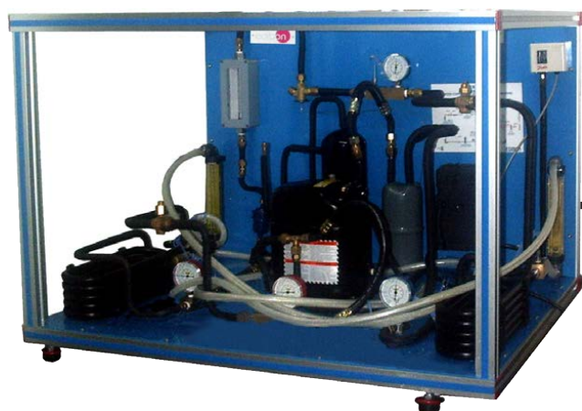
① Unit: THARLLC. Computer Controlled Refrigeration and Air Conditioning Unit (one condenser (water) and one evaporator (water))
