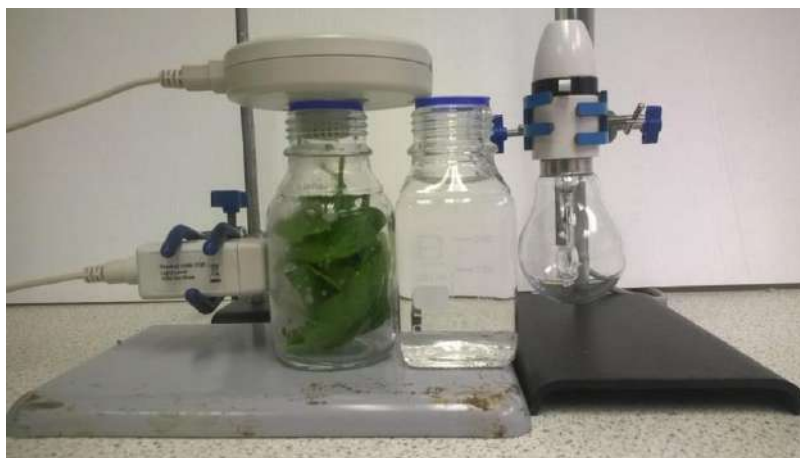
Fig 15b.1 Photograph of typical bench layout of apparatus, the light source would normally be a bench lamp. Note the position of the optional Light sensor.
