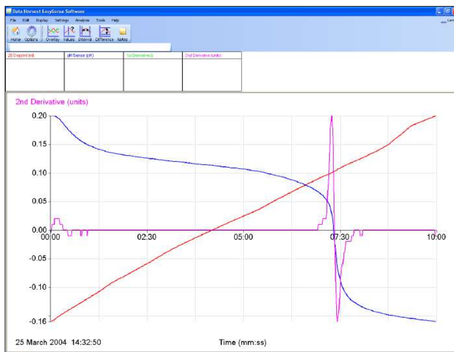
Fig 6.4 Application of second derivative to a titration of sodium bicarbonate with hydrochloric acid, note the intercept of the x-axis.
