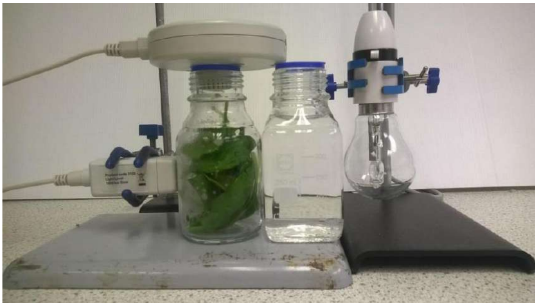
Fig 15c.1 Photograph of typical bench layout of apparatus, the light source would normally be bench lamp. Note the position of the Light sensor.
