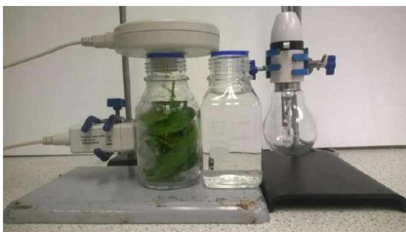
Fig 15d.1 Photograph of typical bench layout of apparatus, the light source would be removed for respiration studies as could the heat sink. We did find that turning the light on was convenient way of bringing the CO 2 levels round the leaves back down to a lower value again.
