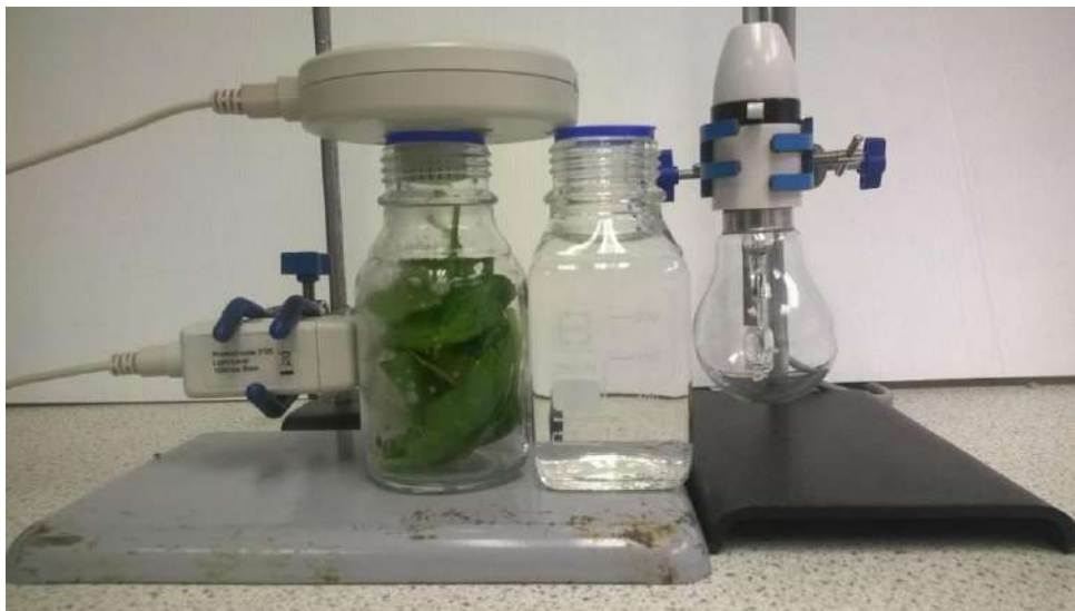
Fig 15d.1 Photograph of typical bench layout of apparatus, the light source would normally be bench lamp. You can use the light source to show the reversal of CO 2 production when light is present.
