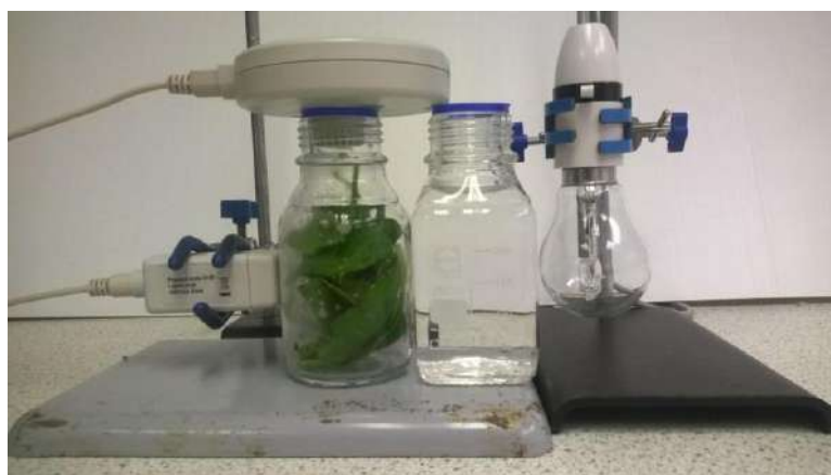
Fig 15a.1 Photograph of typical bench layout of apparatus, the light source would normally be a bench lamp. Note the position of the optional Light sensor.
