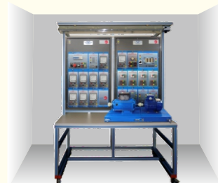
Protective Relays Workbench
