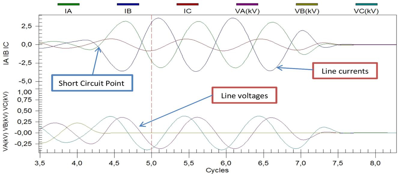
Two-Pole Short Circuit with fault impedance screen
