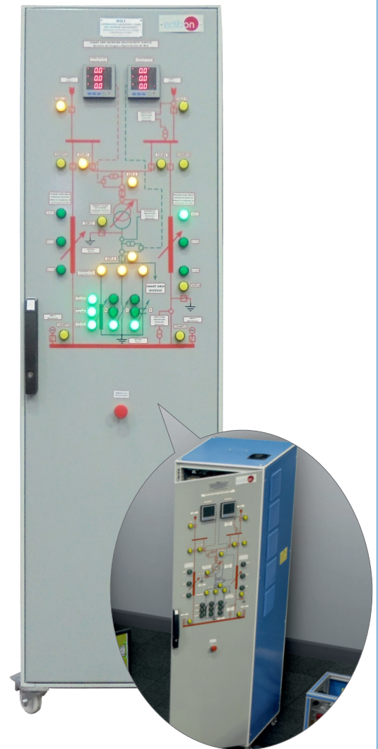
DSL2. Distribution Substation II, Loads and Network Equivalents with Protection Relays System
