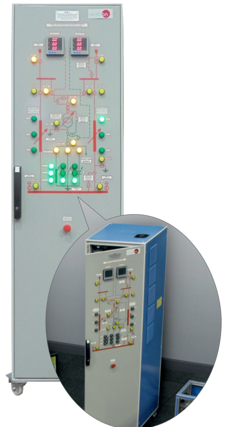
DSL1. Distribution Substation I, Loads and Network Equivalents with Protection Relays System
