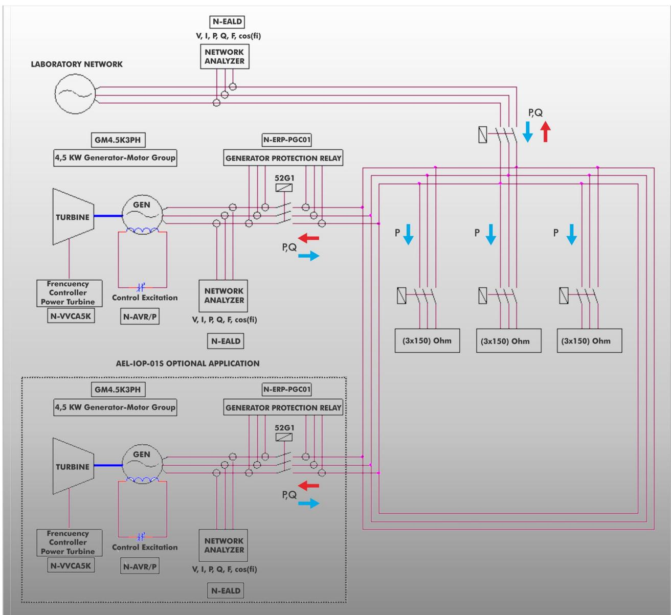
Example of two power generators in parallel operation supplying energy to the loads.
