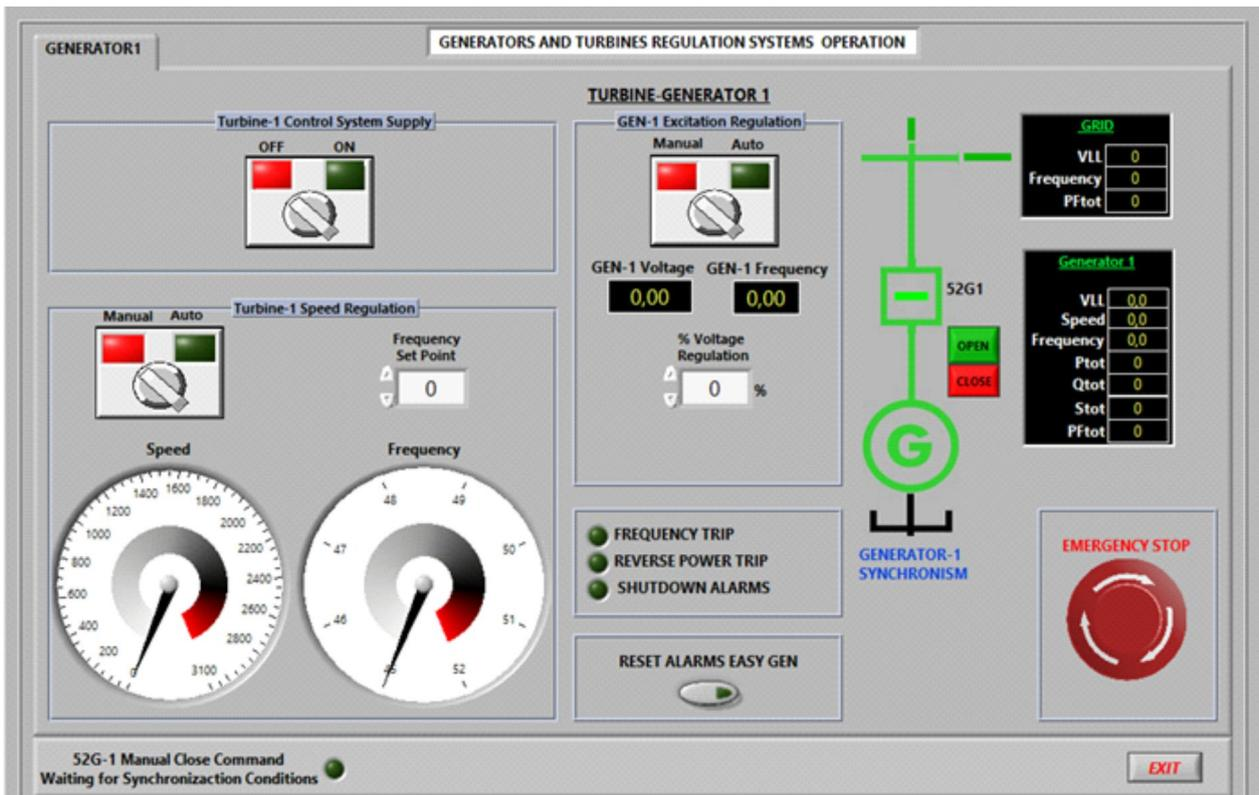
Display control of the turbine and the synchronous generator. This menu offers multiple possibilities for control and regulation of the group.
