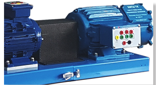
Generator-Motor Group detail
