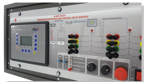
Automatic Voltage and Speed Controller (AVR, ASC) detail
