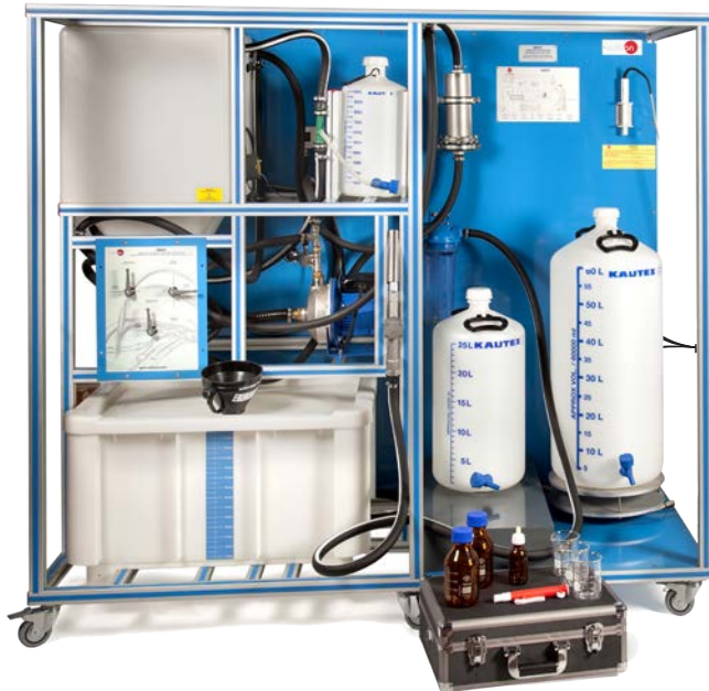
① Unit: EBDC. Computer Controlled Biodiesel Process Unit
