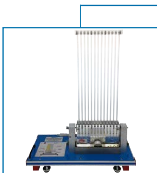
MEMT-1. Radial Pressure Distribution in a Journal Bearing
