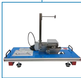
MEMT-2. Dynamic Friction of a Cylinder on a Roller
