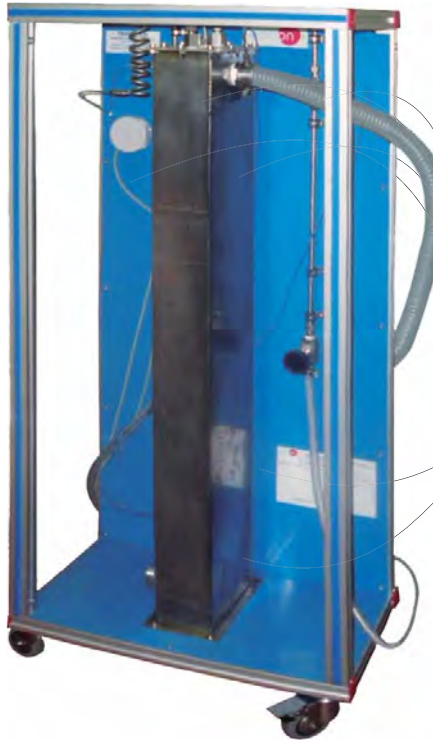
① Unit: TBMC-CG. Exhaust Gas Calorimeter
