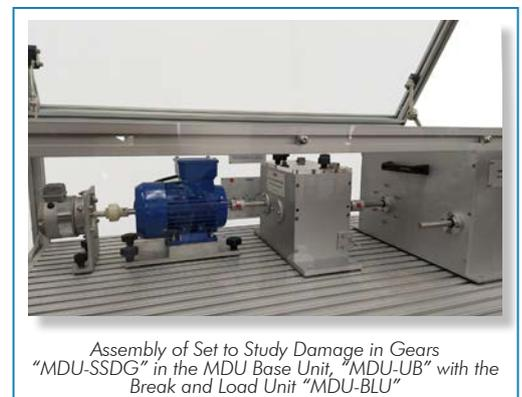
*Assembly of Set to Study Damage in Gears "MDU-SSDG" in the MDU Base Unit, "MDU-UB" with the Break and Load Unit "MDU-BLU"*
